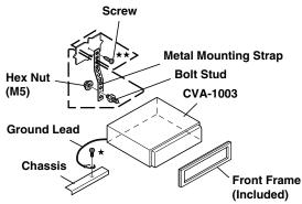
Reinforce the monitor with the metal mounting strap (not supplied). Secure the ground lead of the unit to a clean metal spot using a screw  $(\star)$  already attached to the vehicle's chassis.
